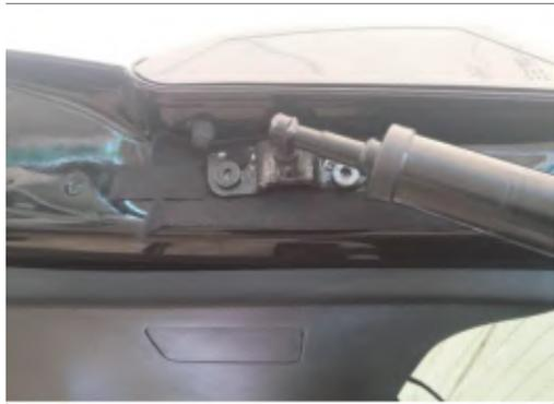
3. Remove the original right support strut and right upper brackets. Then install our upper right bracket.
