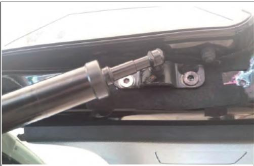
1. Remove the left support strut and left upper brackets of the original car, install our left upper bracket, and fix it with our screws.
