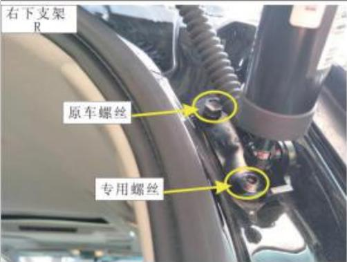
4. Remove the lower right bracket of the original car, install our lower right bracket (ball head facing inside the body) and electric pole, and fix it with the original car screws.
