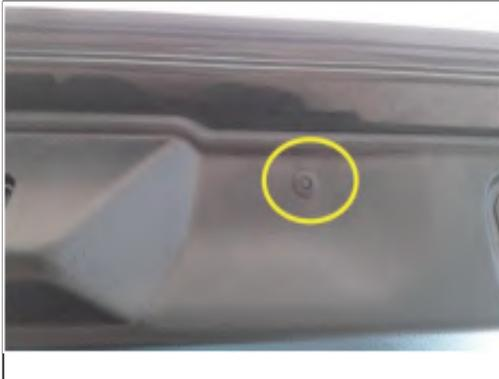
5. Remove the button of the original rear door and remove the trim
