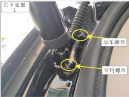
2. Remove the left lower bracket of the original car and install our left lower bracket (ball head facing inside the body) and our electric pole
