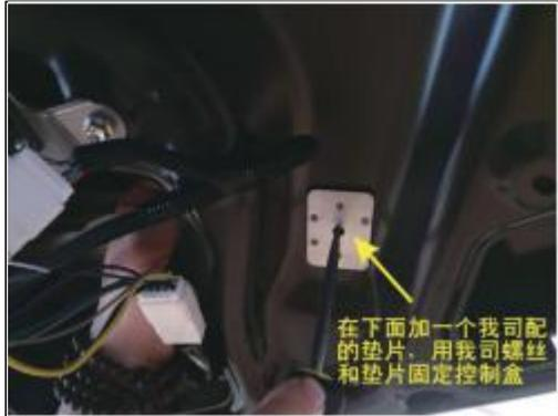
16. Install our control box, add our flat washer under the trim board, and fix them with our screw and flat washer.
