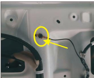
28. Find the original car screw at the tailgate, another cable from the front switch is connected to this screw
