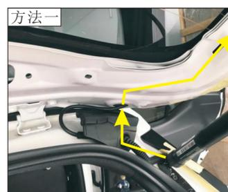
7. The sundial car may try to exit from the threading hole to the tailgate (if it cannot pass through, it can be threaded through the method two holes, the left and right steps)
