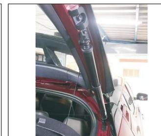
5. The completion of the strut installation
