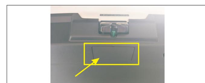
When the tailgate cannot be opened normally, find the original car emergency safety lock in the trunk and open the emergency cover. Pull emergency switch to open
