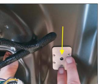
32. Install our control box, add our matching gasket under the panel, and fix it with our screws and gaskets.
