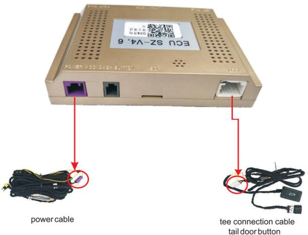
power cable      tee connection cable tail door button
