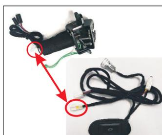
26. As shown in the figure, the socket of the three-way harness is inserted into the power socket of our company.
