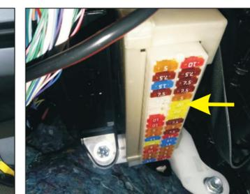
16. Remove the original car yellow 20A fuse under the co-pilot
