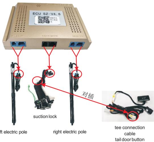
left electric pole      right electric pole      tee connection cable tail door button
