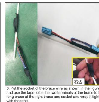
6. Put the socket of the brace wire as shown in the figure, and use the tape to tie the two terminals of the brace to the long brace at the right brace and socket and wrap it tightly with the tape.
