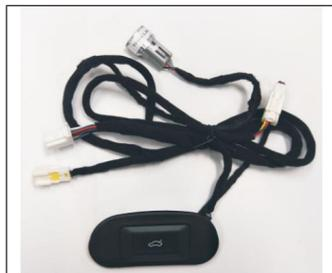
34. Tail door button socket and three-way harness socket plug
