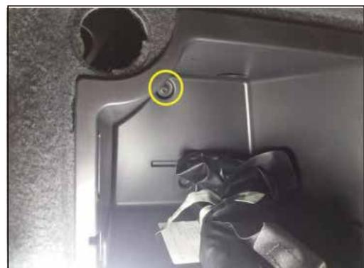
12. After knocking off the screw, the trim board is taken apart to facilitate the placement of our electric suction lock
