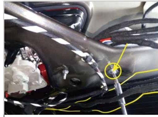
15. Install our central control box here, fix it with our screws, rings and flat washers.
