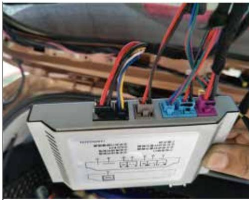
14. Insert the Hall wire, power cord, and electric suction plug into the control box one by one according to the color
