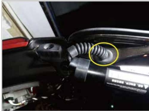
5. The electric pole Hall wire passes through the reserved hole and is plugged with rubber plug as shown in the figure (the left and right steps are the same)
