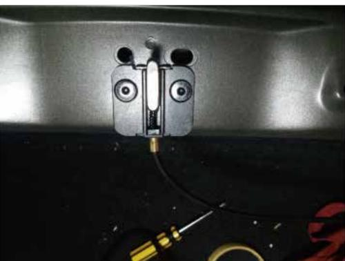
10. Remove the original car lock hook, install our electric suction lock hook, and fix it with our screws.
