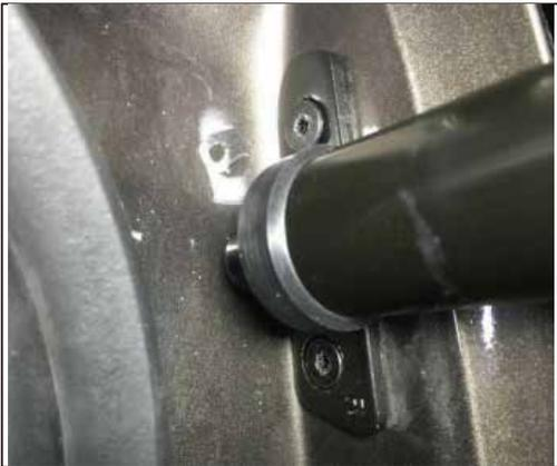
4. Remove the right lower bracket of the original car, install our lower right bracket, and fix the bracket with our screws.
