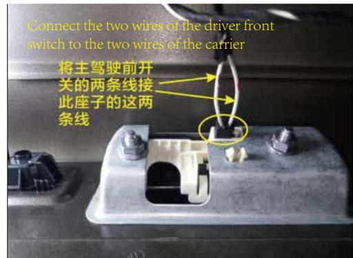
9. Connect the two yellow wires pulled out by the driver front switch to the two wires of the carrier (regardless of direction). This carrier is at the rear trim of the tailgate
