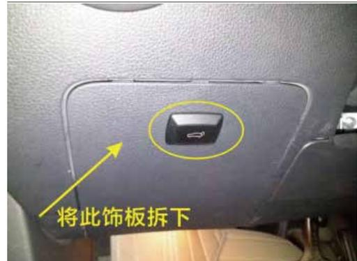
6. Remove the trim board under the main driving, find the power supply, remove the trim board, punch hole and install the front switch
