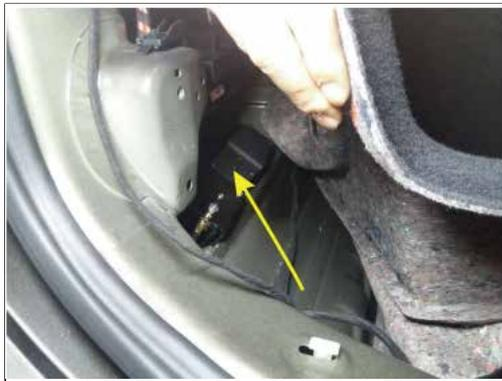
13. The electric suction lock is installed on the right side of the tailgate and fixed with our 3M glue (as shown in the figure)
