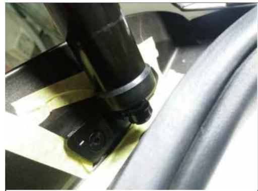
3. Remove the left lower bracket of the original car, install our lower left bracket, and fix the bracket with our screws.
