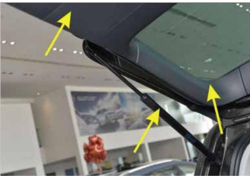
1. Remove the tailgate trim board and the original car support strut
