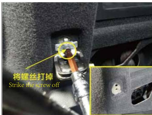
11. Remove the screw on the left side of the trunk and remove the button.
